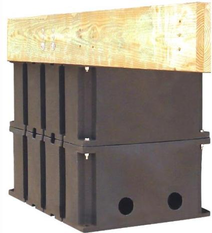
*Wave Defender is composed of a top buoyant float filled with foam attached to a lower, empty, holed float shell (non-standard hole pattern shown here for clarity; wooden stringer not included)*
