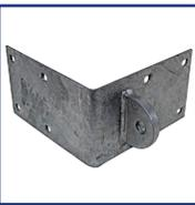
**Outside Corner (male)** - has one 1/2" welded tab. Use with a female outside corner to connect docks end to end. Joint requires 3/4" bolt set or connector pin (L).
