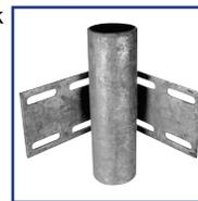
**Inside Corner/Pipe Holder 3"** - these heavy-duty inside corners should be used with one of the outside corners and has an internal pipe holder to be used with 2" pipe. Welded gusset gives strength to the dock's frame. 8-1/4"L x 5"H. Requires carriage bolt set for attaching.
