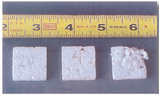
Photo A: Comparison of EPS in AWPA E1 two choice test (4 week exposure) (L-R): PREVENTOL® TM Preservative Insecticide, borate, and untreated.
